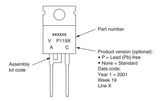
Example: This is a xxxxxx with assembly lot code AC, assembled on WW 19, 2001 in the assembly line "X"
